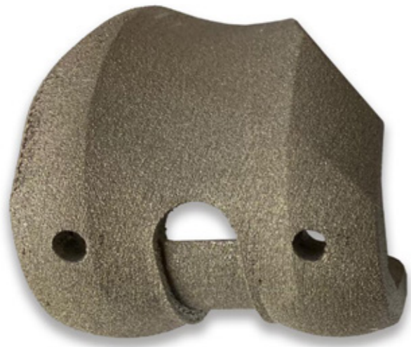
Before Ra 21.02 \mu\text{m}
