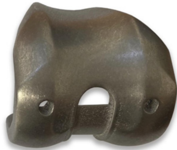
After Ra 3.03 \mu\text{m}
