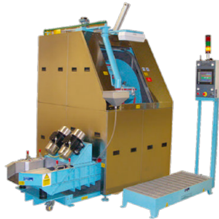
CHE80 with Vibratory Separation System, Platform and PLC
