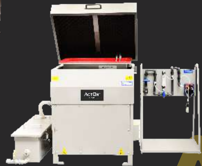
TU3 with dosing unit and settlement tank
