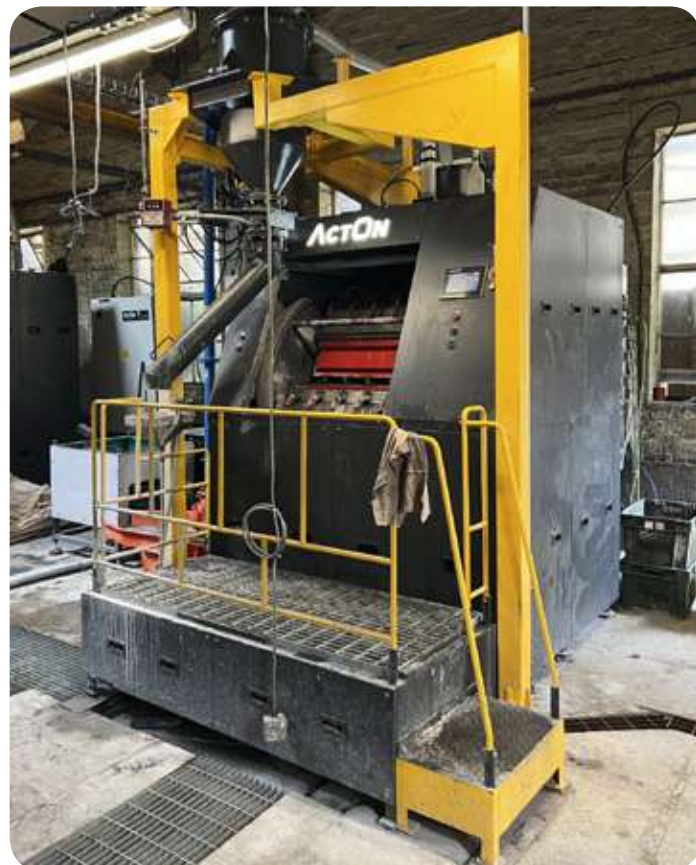
CHE240 with Vibratory Separation System, Platform, PLC, media conveyour
