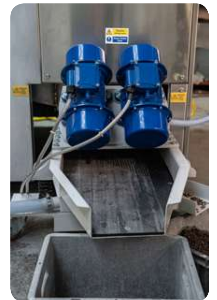
Vibratory Separation System
